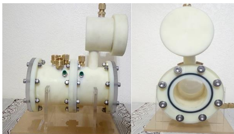
Figure 14. Microbial Electrolysis Cell.
