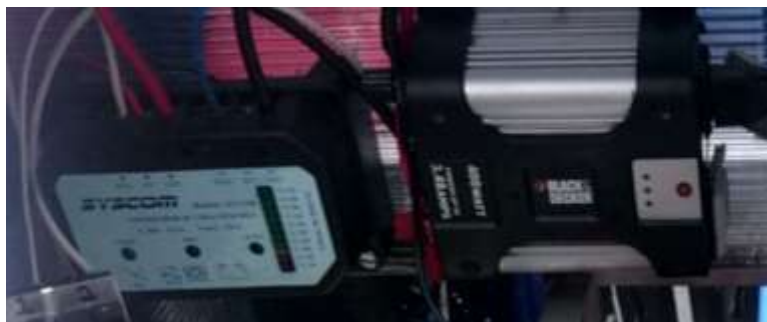
Fig 3. Power Electronics, DC / DC converter and inverter DC / AC.
