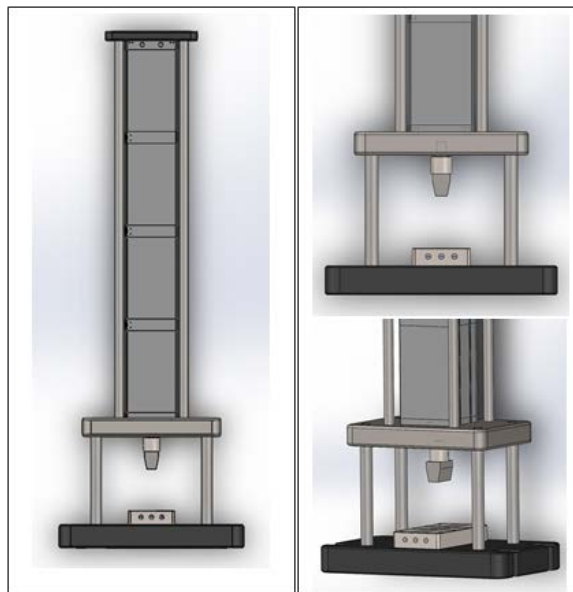
Fig. 1. Front view and some angles of the pneumatic hot-press prototype
