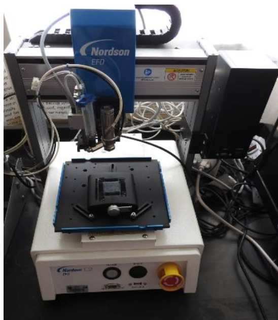
Fig. 2. Left, automatic catalytic ink application system with vacuum table.
