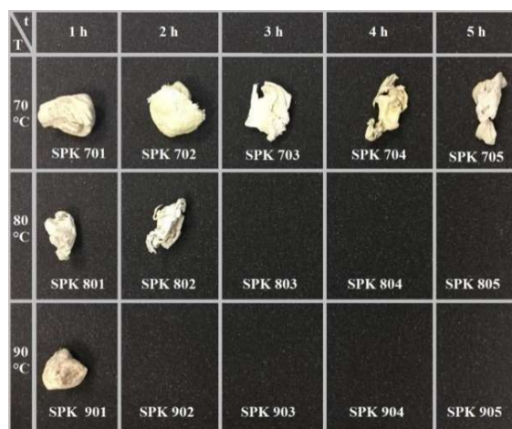
Fig.1 Polymers obtained from sulfonation reactions of PEEK at different time and temperature conditions.
