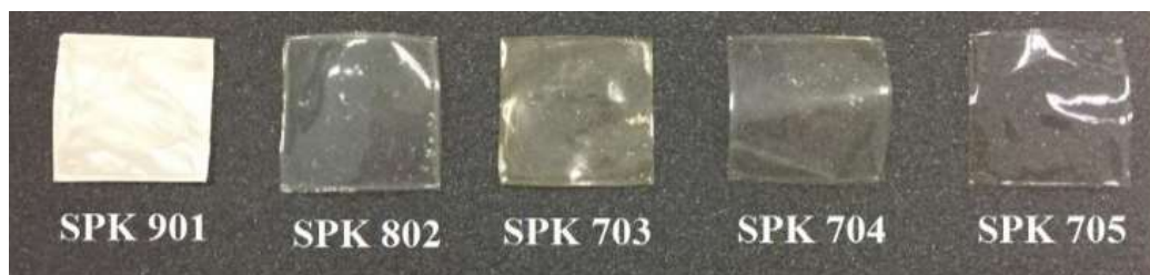
Fig. 7. Membranes obtained with the solvent DMAc
