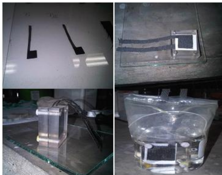
Figure 2. Lab-assembly supercapacitor.
