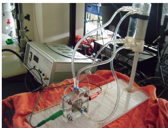
Photograph 9. PEM electrolyzer prototype connected in the table test.
