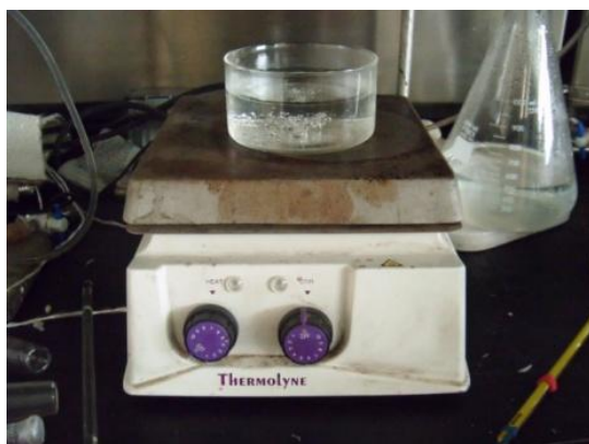
Photograph 1. Activation at 80° for 1 hr.
