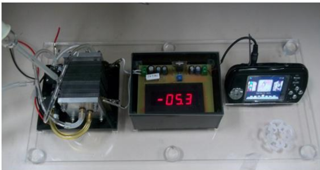
Figure 9. Final prototype of PEMFC stack to charge a MP4 media player.
