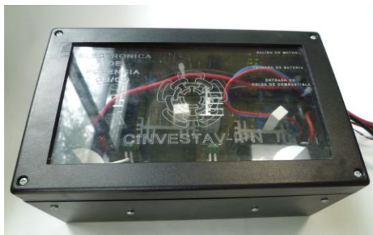
Figure 4. Power Electronics 500W DC / DC converter.
