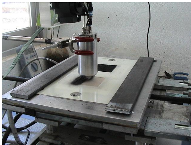
Figure 3. Photography that shows the fabrication of some MEAs using the ultrasonic nozzle.
