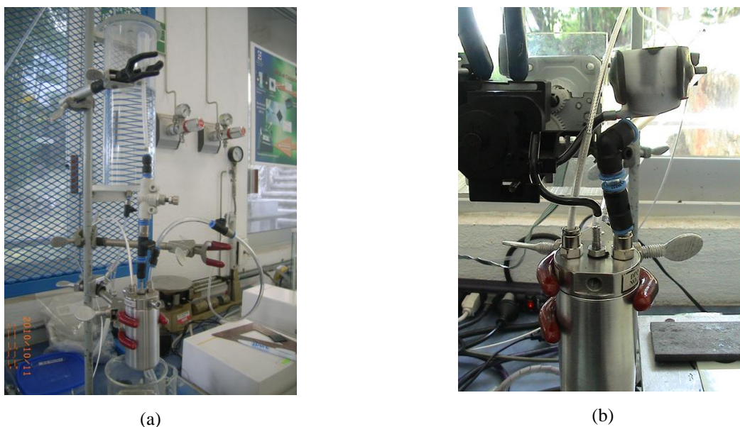
Figure 2. Experimental arrangement for the preliminary tests (a) and the implementation of a small peristaltic pump to manufacture the MEAs (b).
