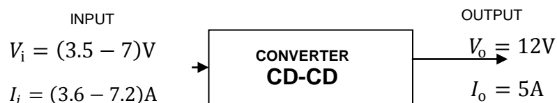
Figure 7. Input and output voltage and current in converter
