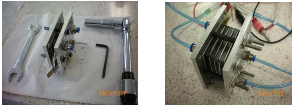
Figure 6. PEM fuel cell assembly and Stack
