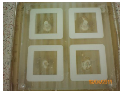
Figure 3. Acrylic mold to make gaskets
