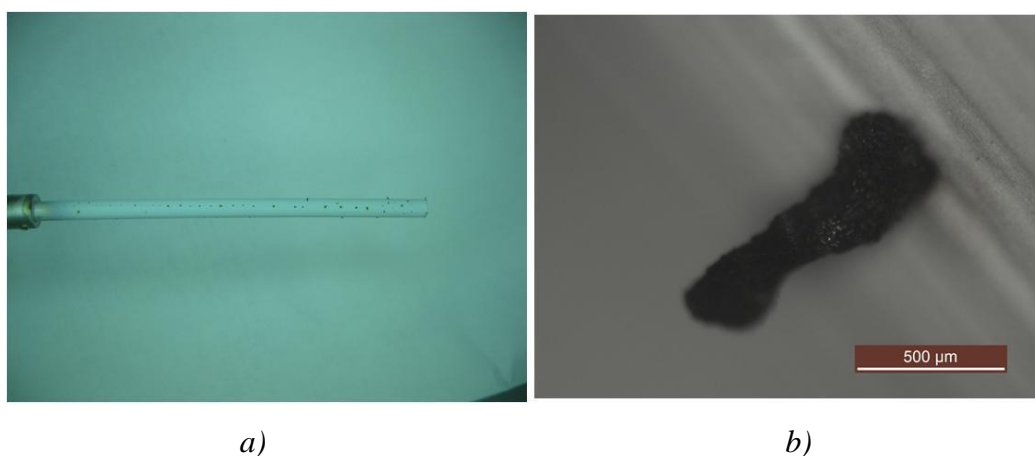
Figure 6. a) Carbon structures found near imperfections on the inner electrode, b) Structures inspected with a stereographic metallographic microscope.
