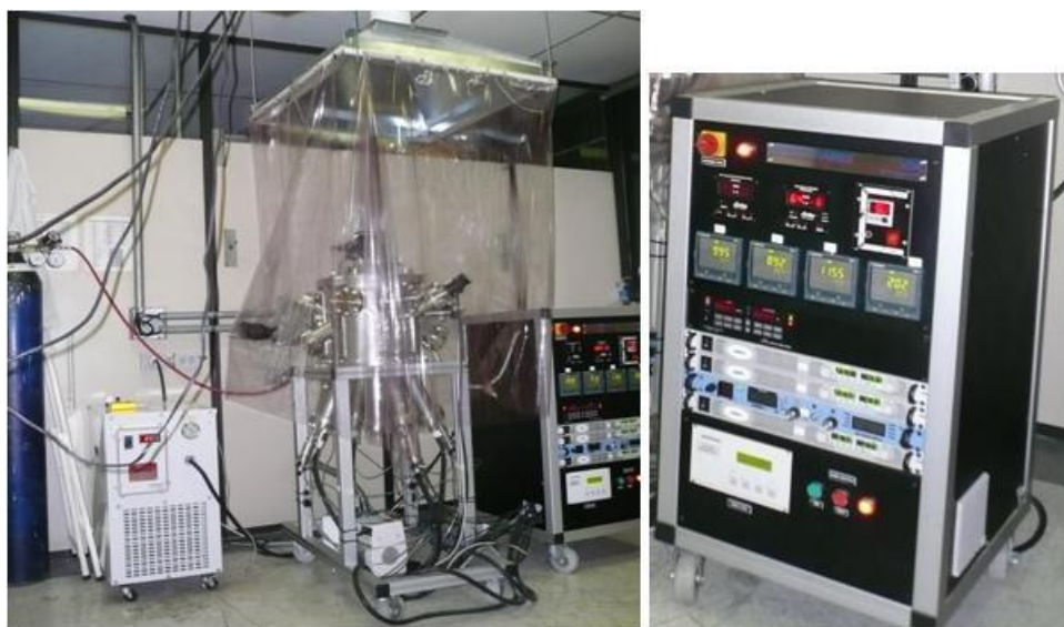
Figure 1. Physical vapour deposition system for co-evaporation of \text{Cu(In,Ga)Se}_2 films. In the left picture it can be seen the vacuum chamber with the four Knudsen-type effusion cells below; the cooling unit is at the left. The right picture shows the control unit.
