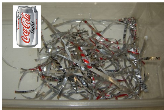
Fig. 1. Al-can and manual cutting to stripes and then to flakes.
