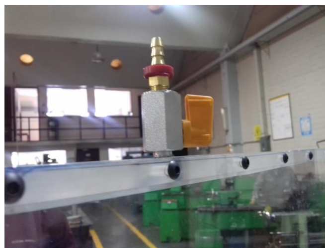
Fig. 5. Valve for gas sampling.
