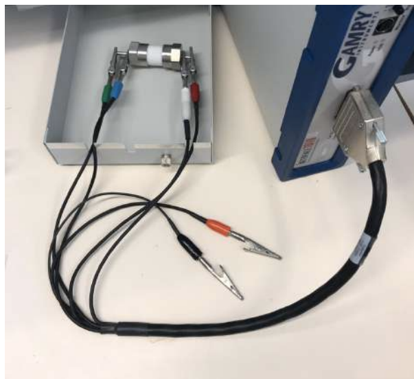
Figure 51. Set up to electrically characterize the supercapacitors.
