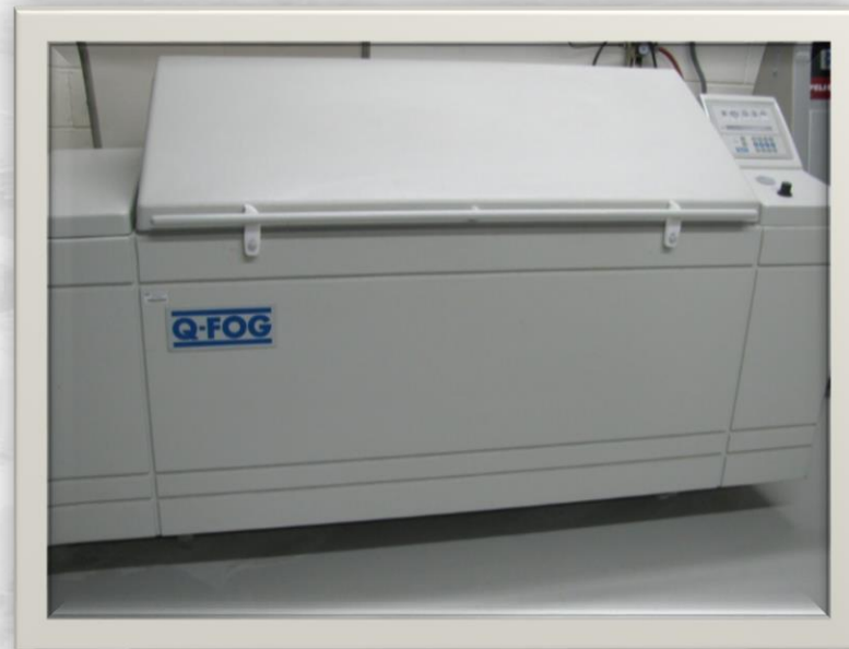
Salt Spray Fog Cyclic Chamber for Corrosion Testing several atmospheres ( O_2 , SO_2 , Cl , etc.)
