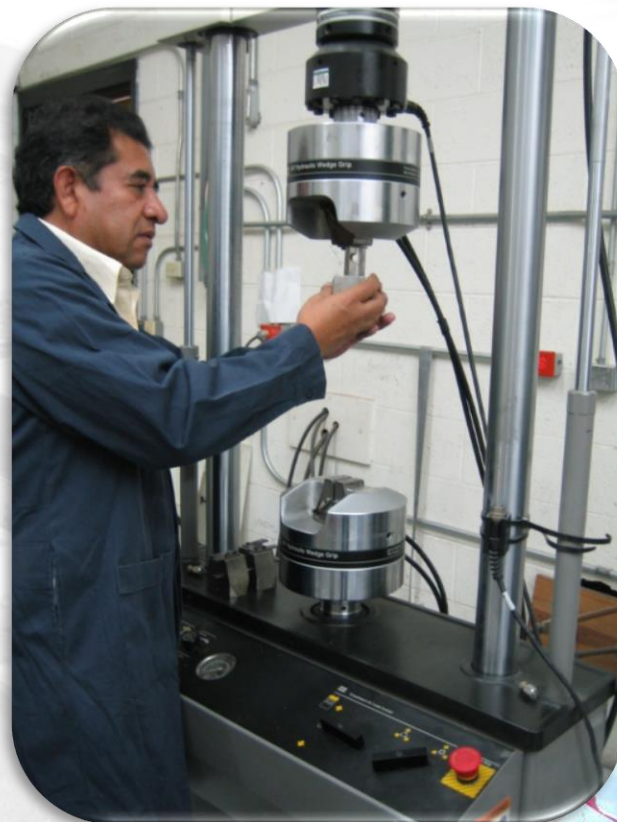
Universal Machines (tension, compression, fatigue). Load capacity: 5,10 and 50 Tons
