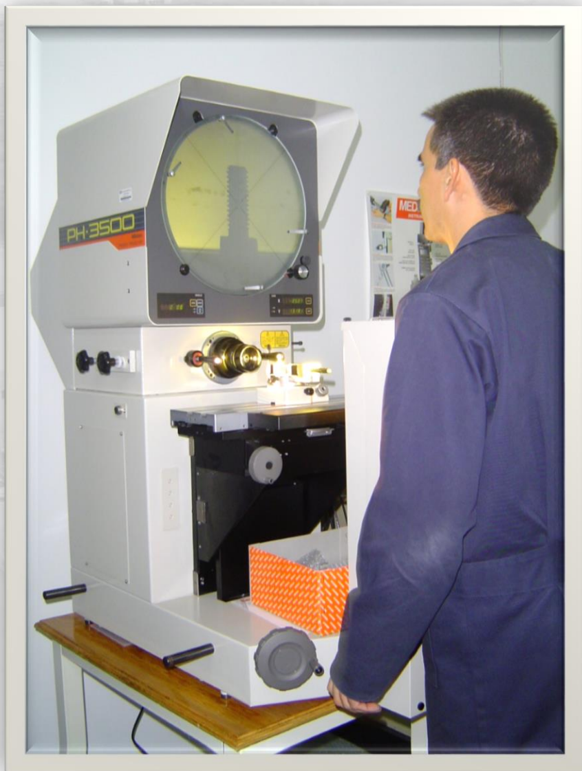
Optical Comparator (Dimensional Measurements)
