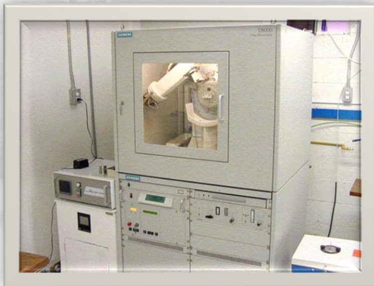
Siemens X- Ray (XRD) (Diffraction (1200°C)
