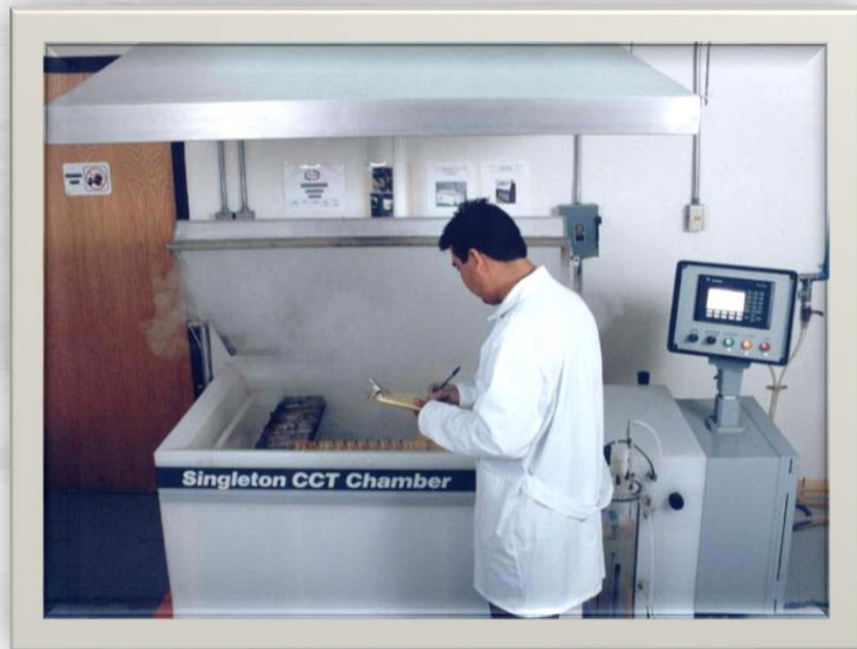
Salt Spray Fog Cyclic Chamber for Corrosion Testing several atmospheres ( O_2 , SO_2 , Cl , etc.)
